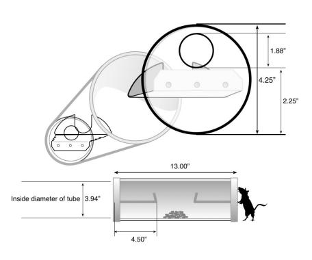
Figure 3. Design of bait stations used to control roof rats and deer mice.
