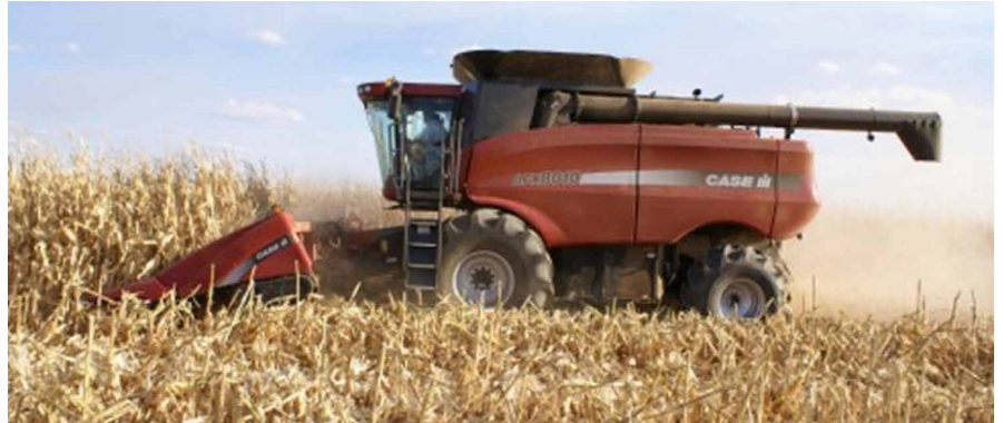
Figure 2: Grain harvesting is normally done with a corn front with either a snapper front or cutter bar (pictured).
