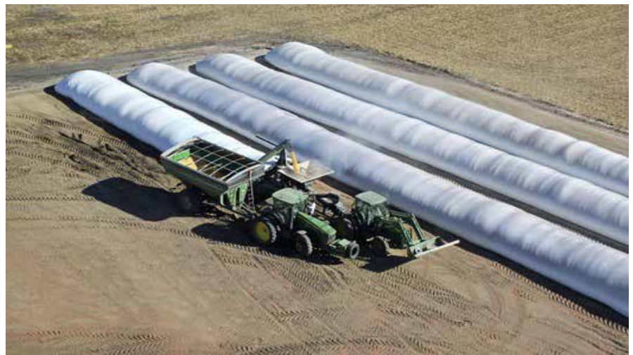
Photo 2: A bag 100 m long can be filled in 30 minutes if there is a constant supply of grain.
