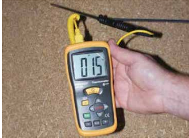
Photo 3: A digital probe is used to check grain temperature and aeration performance.
