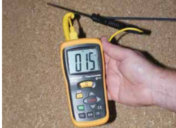
Photo 3: Monitor moisture and temperature using a digital probe from both the top and the bottom of silos, if safe to do so.
