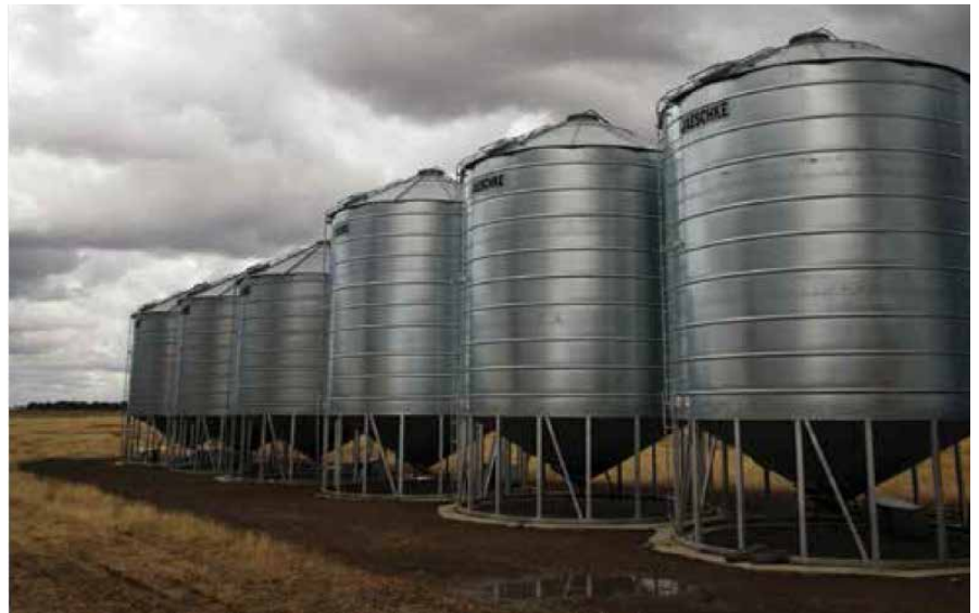
Photo 1: When using on-farm silos it is important to pressure test all silos, even those that are labeled as “sealed”.
