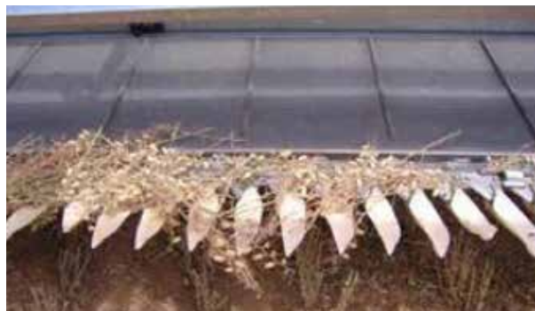
Photo 4: Plastic extension fingers fitted to a draper front.
