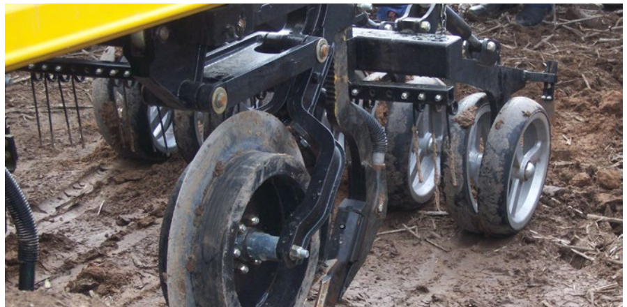
Photo 4: A Bio Blade or Cross slot™ disc opener with opening disc and seeding tine, followed by paired press-wheels. Note that the seed and fertiliser tube has sharp bends and may not be wide enough to avoid blockages while faba bean or broad beans are sown.
