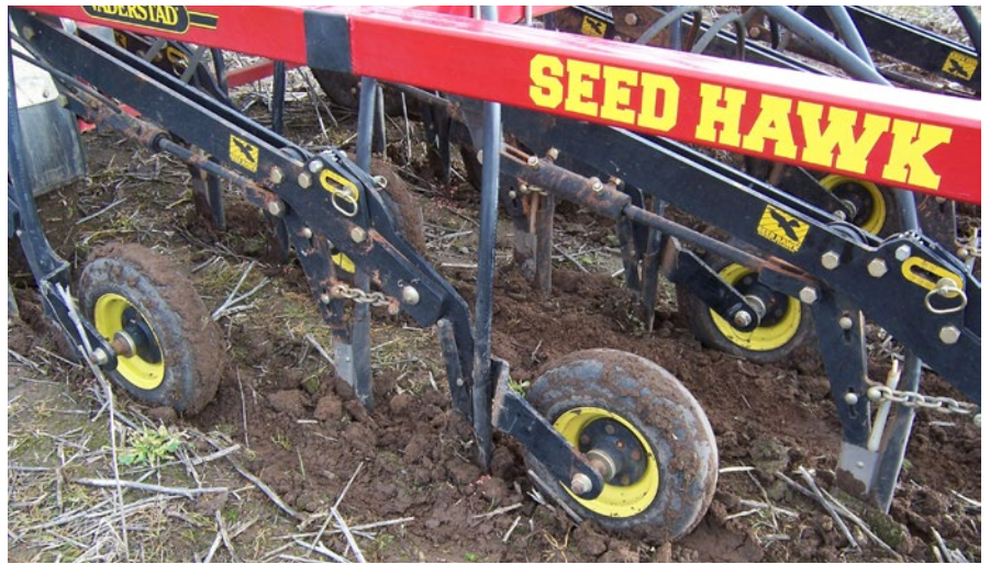
Photo 7: Press-wheels can provide depth control.
