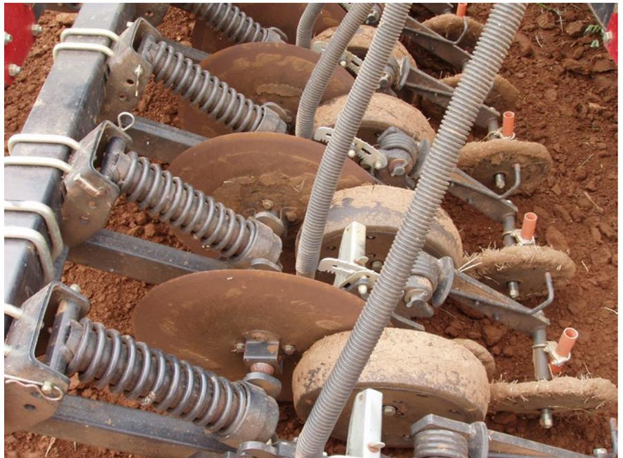
**Photo 9:** A Case IH SDX-40 single disc drill.
