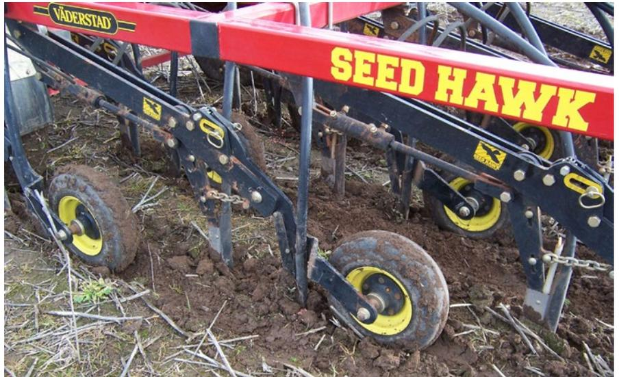
**Photo 8:** One of several seeding mechanisms for uniform seeding depth using the press-wheel for depth control.
