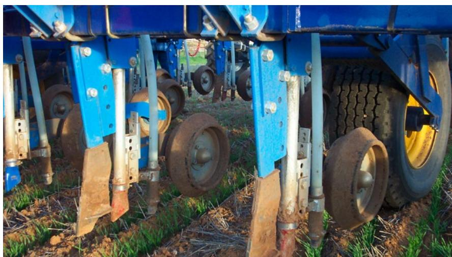
**Photo 5:** A Primary Precision Seeder fitted with hydraulic breakout for consistent penetration. It is also fitted with narrow points that form an 'inverted T' slot. It is capable of deep or side placement of fertiliser.
