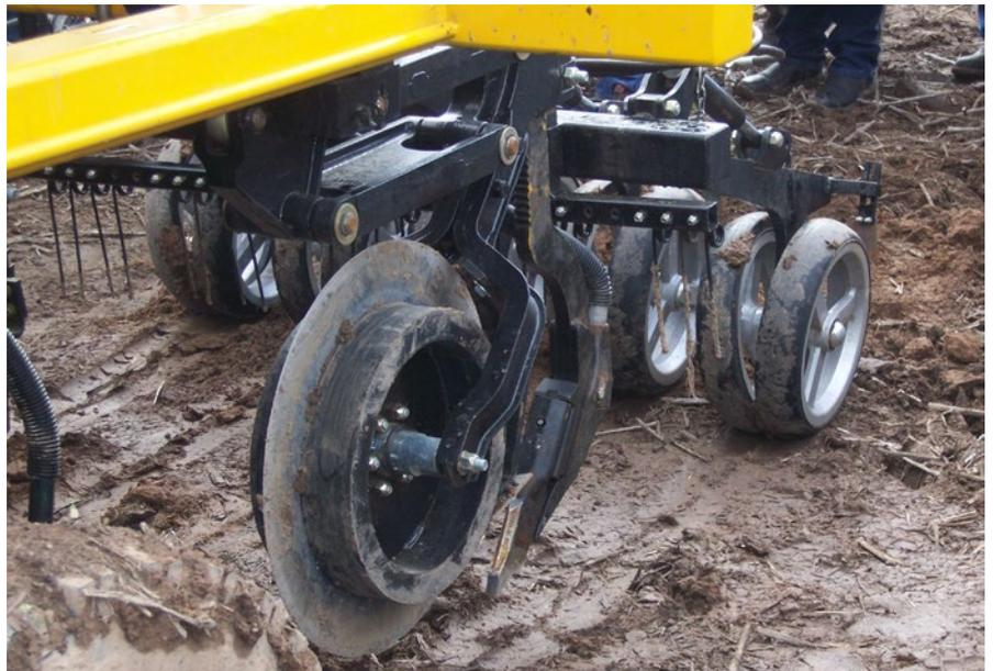
**Photo 7:** A Bio Blade or Cross slot™ disc opener with opening disc and seeding tyne, followed by paired press-wheels. Note that the seed and fertiliser tube has sharp bends and may not be wide enough to avoid blockages when larger-seeded pulses like faba or broad bean are being sown.
