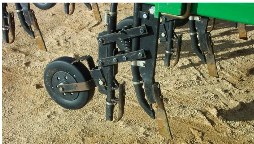
**Photo 6:** The DBS system parallelogram for uniform seeding depth and deep placement of seed or fertiliser.
