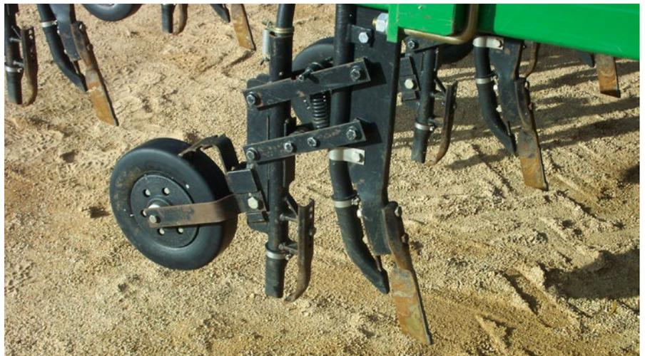
**Photo 6:** The DBS system parallelogram for uniform seeding depth and deep placement of seed or fertiliser.
