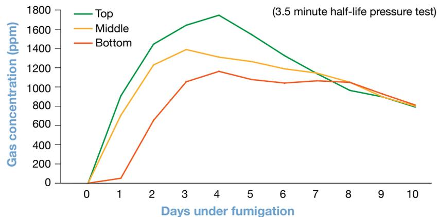
Figure 2: Good gas concentration maintained over time in gas-tight sealable silo. (Source: QDAFF)
