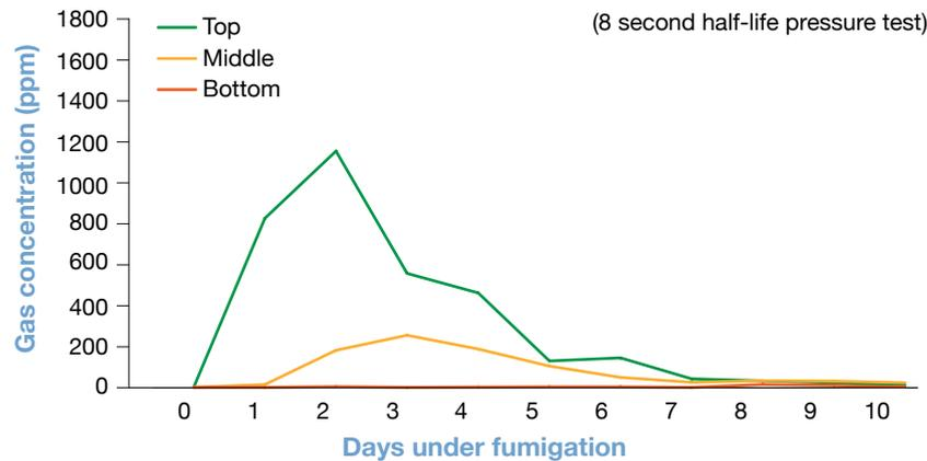
Figure 3: Gas concentration is poor over the 10 days in a non-gas-tight silo. (Source: QDAFF)
