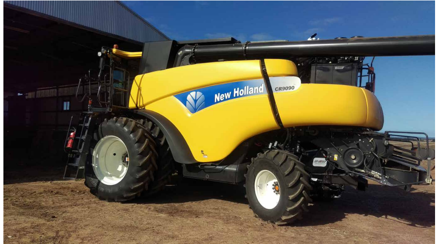
Photo 6: Integrated Harrington Seed Destructor.
