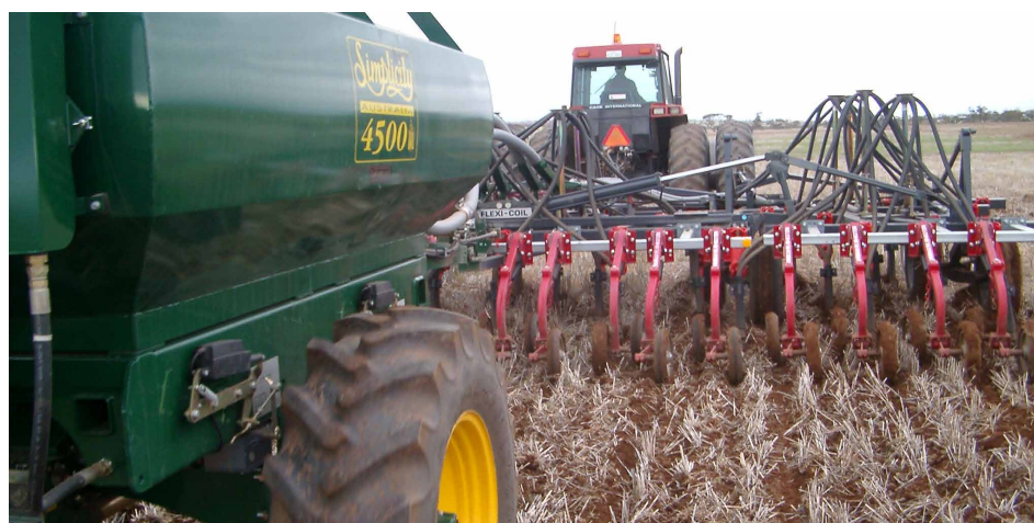
Figure 14: Seeder calibration is important for precise seed placement and seeders need to be checked regularly during sowing. (Photo: Rohan Rainbow)
