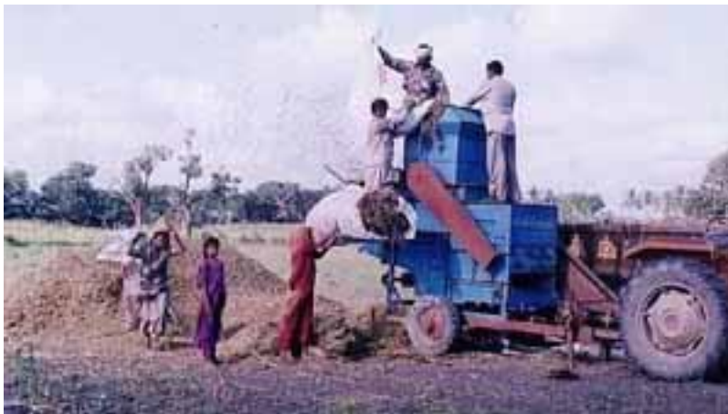
Figure 12: Threshing operations in the field, groundnut opener being operated with the help of tractor engine and another with a diesel engine.
