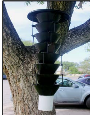
Figure 9. A Lindgren funnel trap with a lure to attract the walnut twig beetle. The insects impact the funnels when flying to the trap and are collected in the cup at the bottom.
