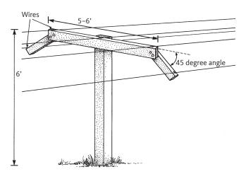
Illustration 1A. Standard T-bar trellis system for kiwifruit
